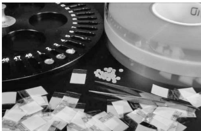
Figure 3.9 Available forms of \text{Al}_2\text{O}_3\text{:C} detectors, including round single crystals \sim 5 mm in diameter by 0.9 mm thickness, 0.3 mm thick tapes containing a detector layer consisting of \text{Al}_2\text{O}_3\text{:C} powder and organic binder, and pieces of tape of sensitive area \sim 1.7 cm \times 2.0 cm used in the Luxel dosimetry system (Luxel detectors).
